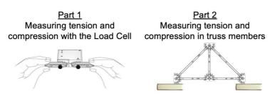
The load cell allows students to immediately experience the relationship between a force tension or compression - and the positive or negative value that describes that force. Pushing on the load cell creates a compression or negative force. Pulling creates a tension, or positive force. The human brain is a master of visual processing. Visualizing abstract ideas is a powerful way to create real and lasting understanding, a central goal of teaching and learning.
